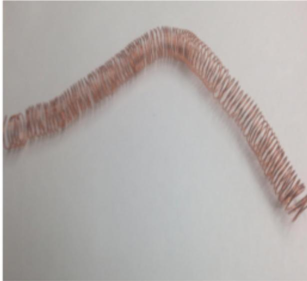
Figure 7: Finished Solenoid
