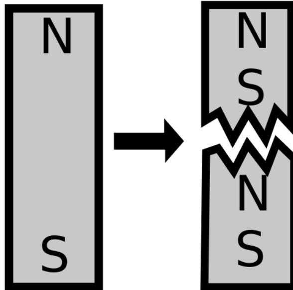
Figure 4: Magnetic Dipoles
