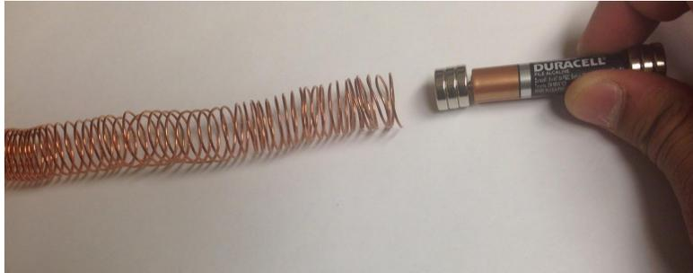
Figure 1: Finished Solenoid Track and Battery Train
