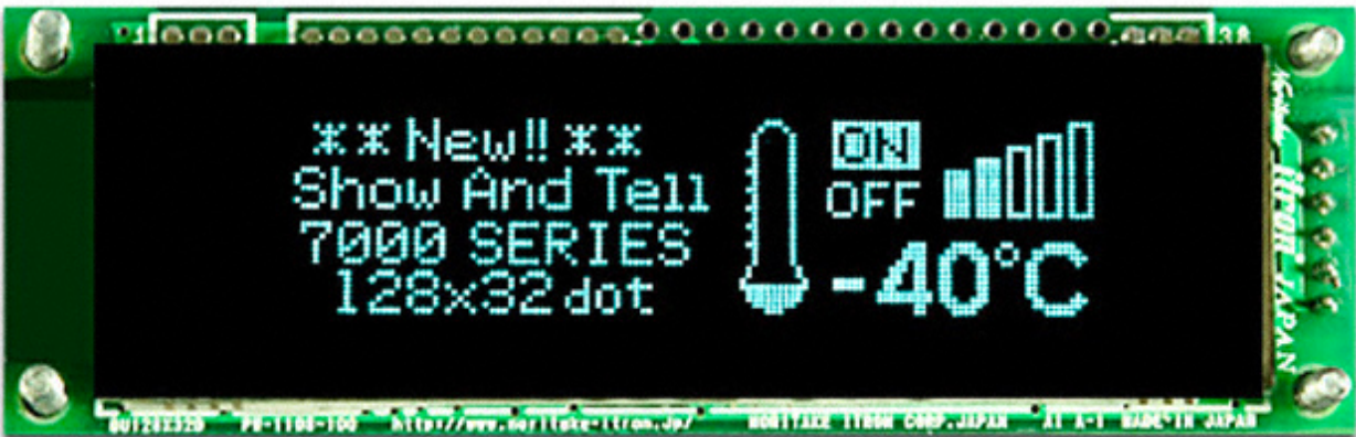
The vacuum fluorescent display
