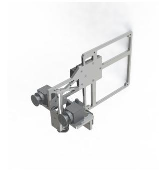
Fig. 6. Close-up of a CAD rending of motherboard mounting system, with cameras in place.
