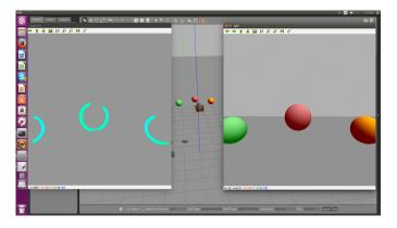
Fig. 7. Example of simulating the stereo camera system in Gazebo. Pictured is a disparity image (left), the simulated scene (center), and the raw image from the simulated left camera (right).
