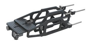
Fig. 4. CAD rendering of Riptide's previous electrical mounting system.
