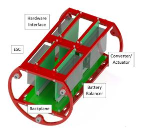
Fig. 6. CAD rendering of the internal electronics.
