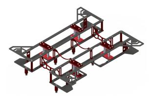
Fig. 3. CAD rendering of Puddles' chassis.
